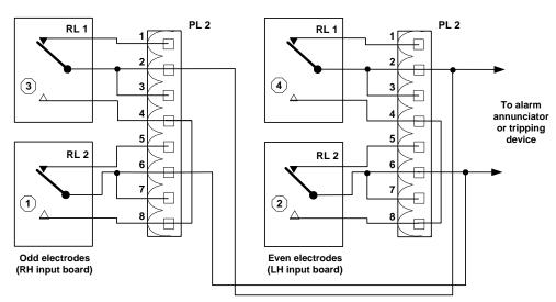
Case B - Relays normally de-energised, energise one in each pair to trip (Relays shown in de-energised state)
